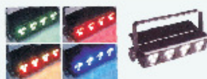
LW-240-PC-W LED WALL WASHER (II) - one row, for outdoor use (IP65), 240V, 12pcs 1W high power white leds, max power consumption: 30W, weight: 1,5kg
